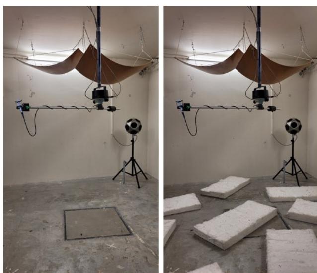
Figure 1: Measuring room. (Left: RT_{\text{average}} = 4 s; Right: RT_{\text{average}} = 1 s)
