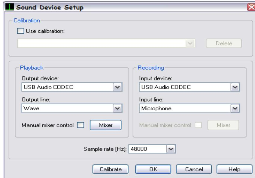
During the calibration procedure, Dirac finds the optimum settings for all relevant volume controls, and the optimum DAC levels. Also, the frequency response of the sound device is measured and, if needed, used to compensate the measurements.
