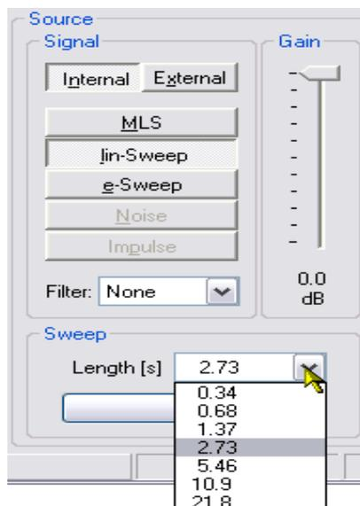
The length of the generated signals can be set through the signal **Length** drop down list box.
