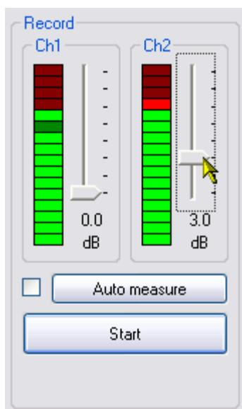
The third section of the measurement window (**Record**) is used to check the recorded signal strength and to start a recording. The recording level can be adjusted using the **Ch1** and **Ch2** gain sliders. Each element of the level meters represents a 3 dB signal level range. The gains should be set such that the level meters reach the topmost green levels. This allows for a 12 dB headroom.
