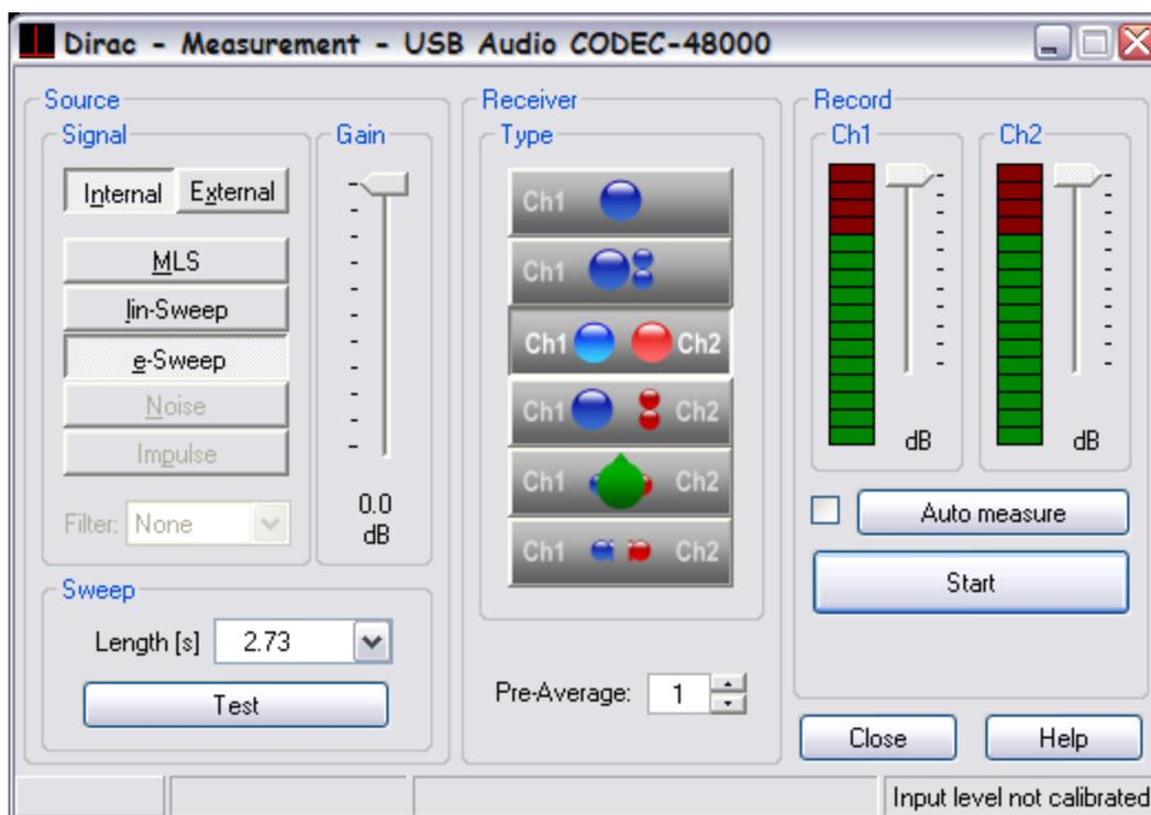
The measurement window consists of 3 sections: Source, Receiver and Record.
