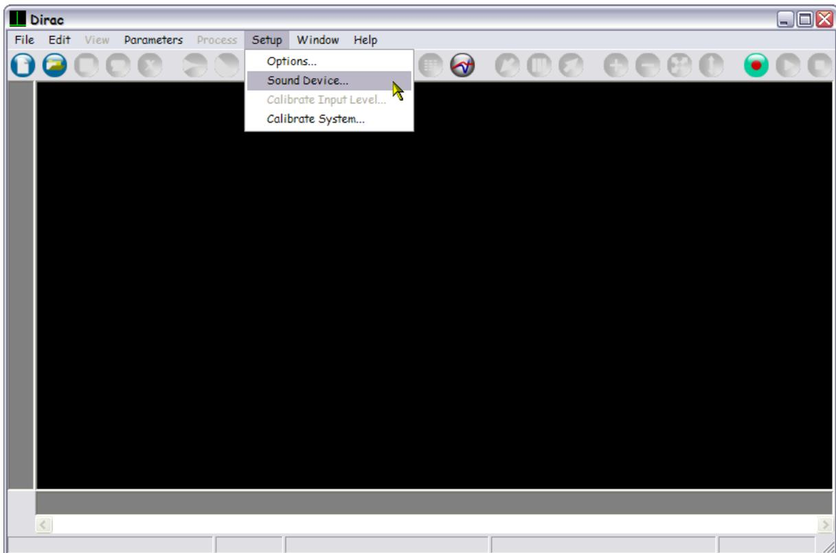
Initially, Dirac will use the default sound input and output lines used by Windows. In the **Sound Device Setup** dialog you can select the device you wish to use for the actual measurements. For optimum performance and full control of the sound device by Dirac, you should perform the calibration by clicking the **Calibrate** button and following the ensuing instructions.
