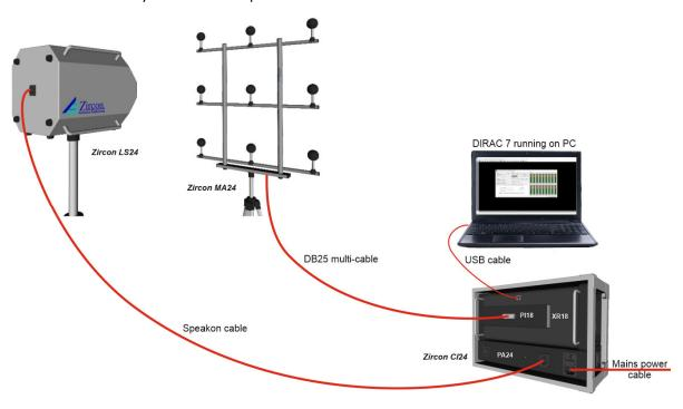
Dirac 7 running on the PC will generate a stimulus signal that is sent to the CI24 which acts as a sound device for Dirac. The CI24 amplifies the signal and sends it to the LS24 loudspeaker. The emitted (and reflected) signals are picked up by the 9 microphones of the MA24 microphone array, and amplified and sampled by the CI24. Dirac 7 then processes the signals captured by the CI24 into impulse responses.
