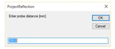
When you start the script you will first be prompted to enter the distance between the microphone array and the surface under test in mm.
