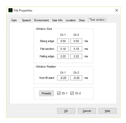
To set another time window, modify the values on the **Time window** tab, or select a preset time window. To apply the preset to both channels, make sure that the check marks for CH1 and Ch2 are set. Then click **Presets** and select one of the preset windows.
