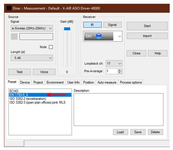
Note that the **loopback channel** is set to 17. This guarantees accurate source-receiver distance measurements.
