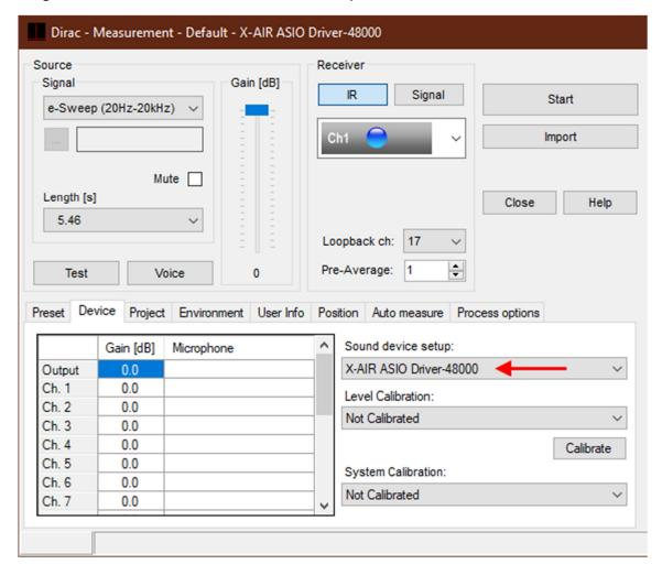
Note that no level calibration is required for this type of measurement because the reflected signal is compared with the free-field signal and only their relative levels are important.
